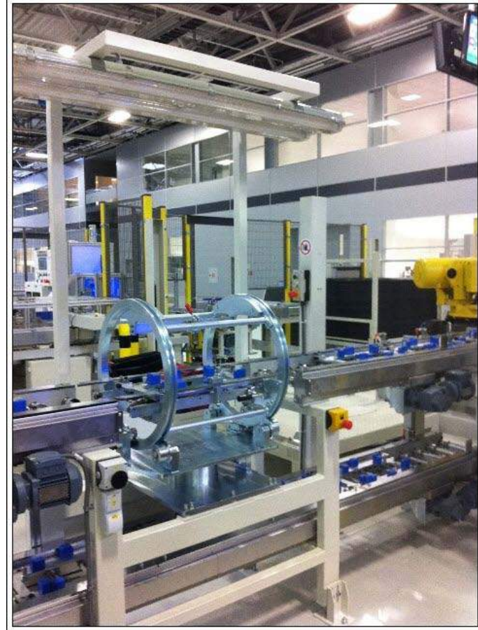
HEAD INSPECTION CONVEYOR
